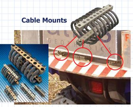
Cable mounts are designed to perform efficiently without material or performance degradation in extremely hostile environments. They are operational under wide extremes of temperature ranges and resist chemicals, oils and abrasives.
