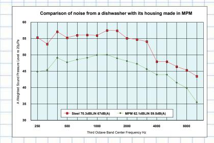
Noiseless Metal is used in computers, printers and other office machines in which damping of structure-borne sound is essential. Even the quality of record players and loudspeaker units has been considerably improved by using NM panels in their construction. Where domestic appliances are concerned, the structure borne sound damping properties of NM are used for damping the noise from dishwasher cabinets and other kitchen equipment.
