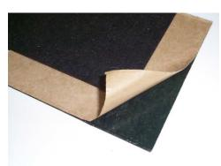
**DBL Damping Sheets** (*DBL*) is a self-adhesive, lightweight damping pad material used for controlling noise and vibration in truck, bus and industrial machine sheet metal applications. The pad material is odorless, wear resistant, and waterproof. DBL provides damping performance equal to that of conventional materials twice its weight.
