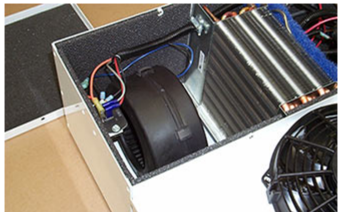
Foam damping sheet placed inside air conditioning unit for heavy equipment cab.
