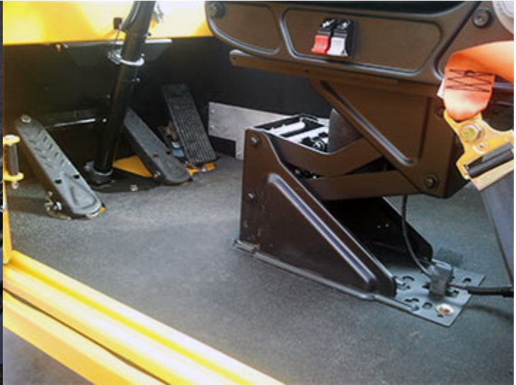
OEM Lava style floormat installed in new terminal tractor.
