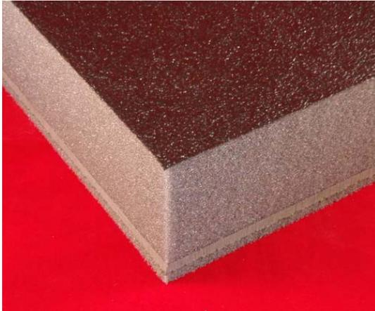
**Whispermat WM2-24-2.00A-BU** is a special barrier absorption composite which combines a urethane film for liquid resistance, a two inch thick polyurethane foam for sound absorption, a loaded flexible 1.6lb/ft<sup>2</sup> barrier on a ¼" thick polyurethane foam de-coupler for sound transmission loss.
