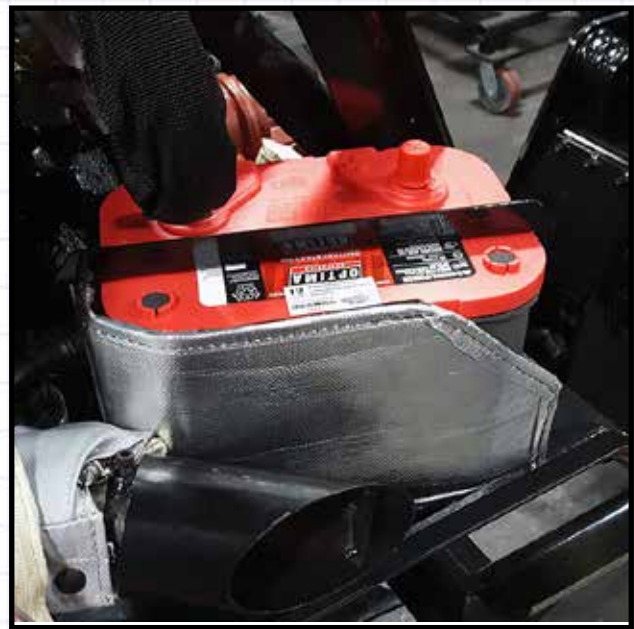
This heat shield protects the battery in a diesel engine compartment.
